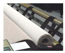
IMPORTANT NOTE: IF YOU CONTINUE THE ROLL-UP PROCEDURE BY PRESSING THE JOG BUTTON INSTEAD OF THE FOOT SWITCH TAPE, THE MACHINE WILL NOT STOP AUTOMATICALLY AT YOUR PRE-SET LENGTH. BE SURE TO USE THE FOOT SWITCH TAPE AFTER YOU HAVE STARTED THE CARPET SO THIS FUNCTION CAN PERFORM PROPERLY.
