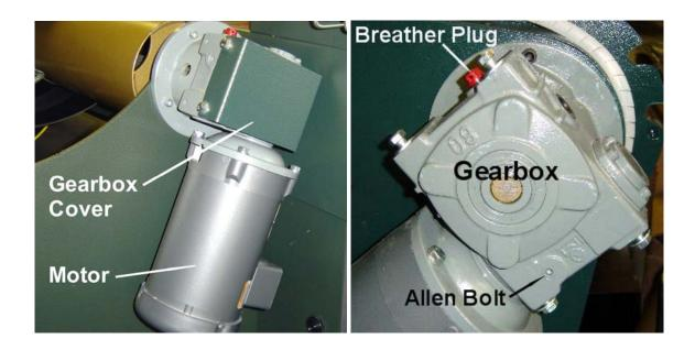
Use 9 to 11 ounces of oil per gearbox for your MK-100. Due to the mounting configuration, the window on the gearbox cannot be used to monitor the amount of oil however you must ensure that the gearbox is <u>never more or less then half filled with oil at all times!</u> Quaker State Synthetic Gear Oil is recommended but any brand between 75W to 90W Synthetic Gear Oil or Synthetic High Pressure Gear Oil is acceptable.
